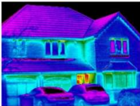
If you have cavity walls, insulate them. This house is Grade A
